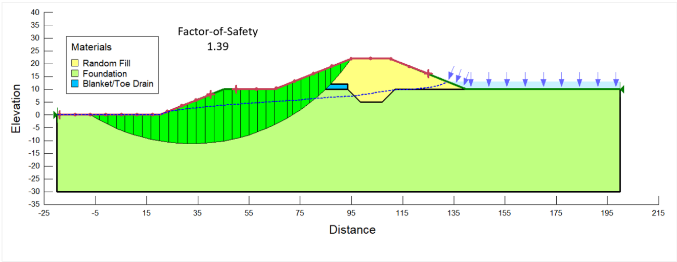
Figure E-15. Levee embankment slope stability for 12-ft-high option with toe loaded to steady-state condition and OBE (0.07g) seismic load applied.
